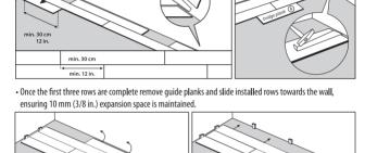
A 10 mm (3/8 in.) expansion space must also be maintained around plumbing, pipes and any vertical objects. If fitting planks around plumbing, cut holes approx 20 mm (3/4 in.) larger than the diameter of the
